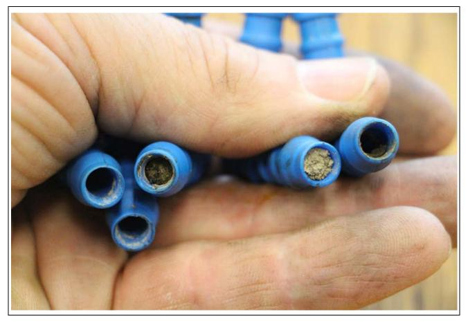
Vacuum action distributes fine particles throughout the entire system. This in turn gave rise to defects on the couplings that then developed leaks. A small lack of attention to detail when working with a vacuum lifting device therefore gave rise to a relatively significant damage incident.
