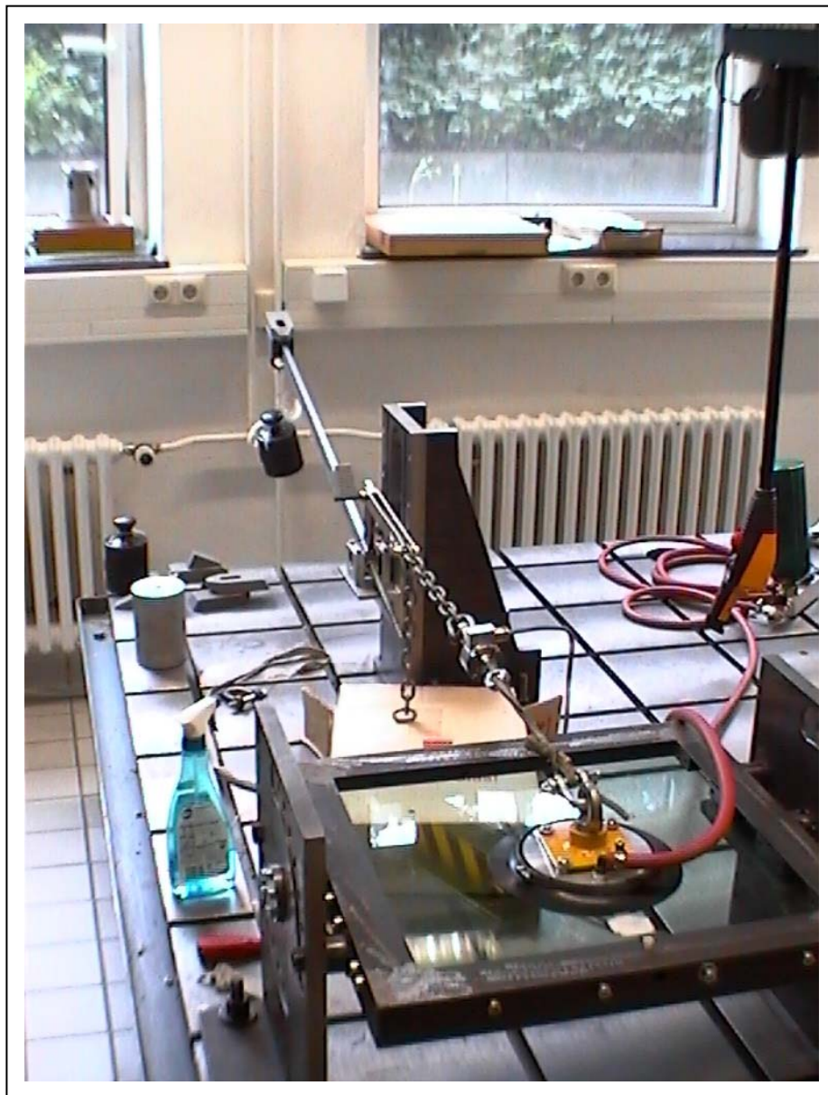
Picture 1: Test construction for static suction cup test, here with suction cup Euro-Tech 540
