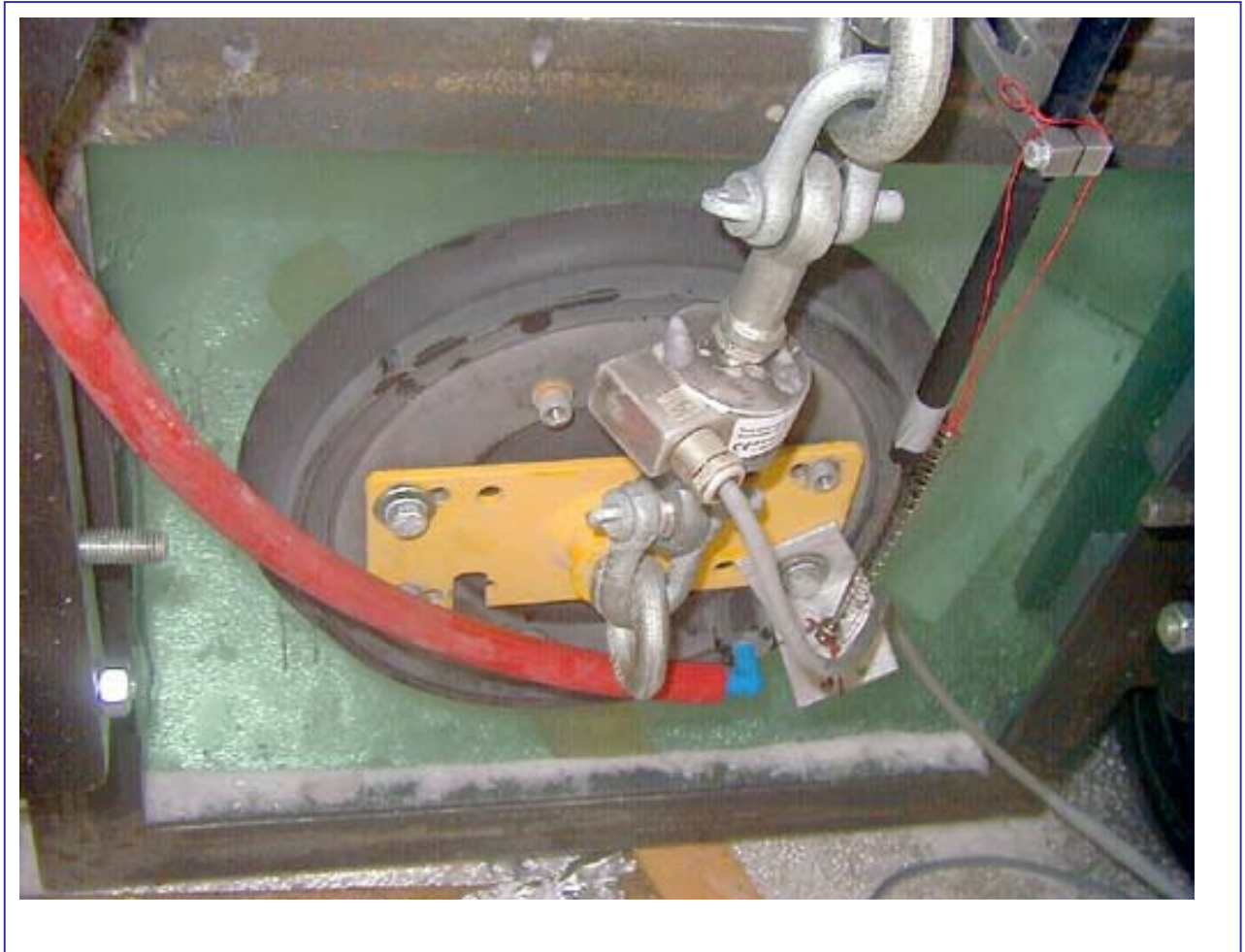
Picture 3: Suction cup 388 at -32.1\text{ }^{\circ}\text{C} . The suction cup doesn't pull in spite of powerful surface pressure
